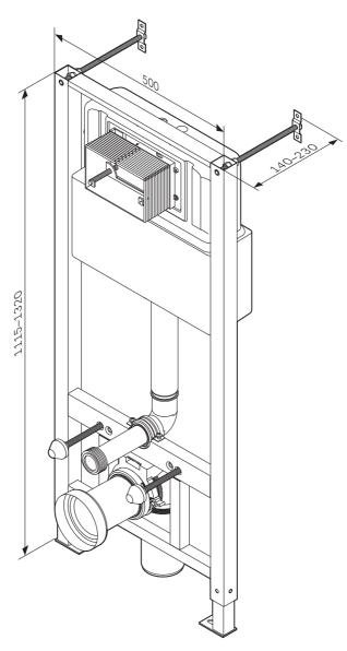
ENG Installation system for wall-hung WC with control panel
